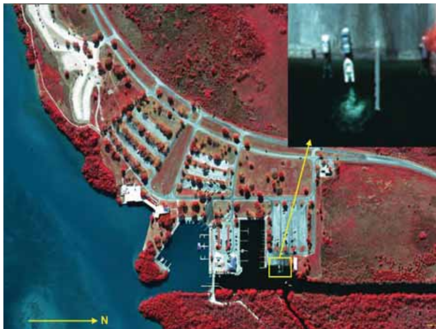
FIGURE 8-63. AN EXAMPLE OF A COLOR INFRA-RED COMPOSITE OF DIGITAL AERIAL PHOTOGRAPHY LOCATED AT THE FLAMINGO MARINA IN EVERGLADES NATIONAL PARK WITH THE ENLARGEMENT SHOWING A BOAT BEING LOADED ONTO A TRAILER AND THE BOAT'S PROP WASH
